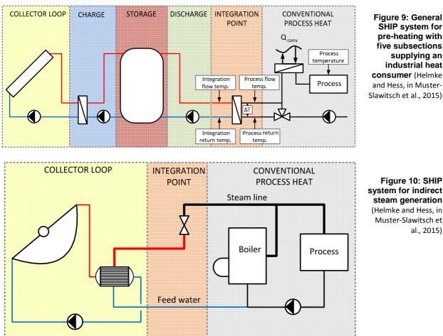
SHIP system for pre-heating with five subsections supplying an industrial heat consumer (Helmke and Hess, in Muster-Slawitsch et al., 2015)
