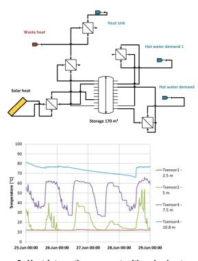
Figure 2: Heat integration concept with solar heat and simulation result of a combined storage (Krummenacher and Muster-Slawitsch, 2014)
