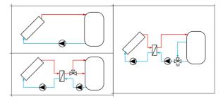
Figure 4: Different charging concepts ((a) direct charging without heat exchanger; (b) external heat exchanger with stratification valve; (c) external heat exchanger with mixed charging return flow) (Helmke and Hess, in Muster-Slawitsch et al., 2015)
