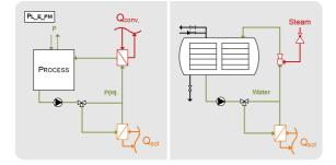
Figure 3: Integration concepts for direct solar steam generation (above) and solar heating of a product or process media with external heat exchanger (below) (Schmitt, in Muster-Slawitsch et al., 2015)
